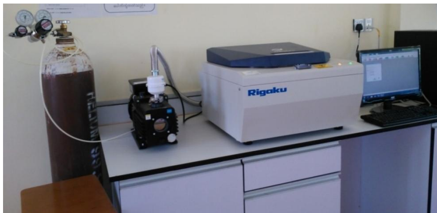
Figure 6 Experimental Set-up for Energy dispersive x-ray fluorescence spectrometer (Rigaku) in University Research Centre, Taunggyi University
